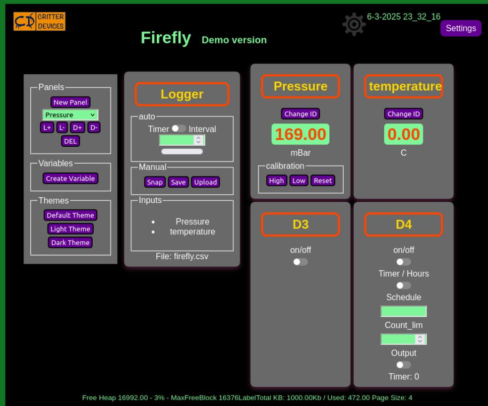
In the above picture I have already selected the temperature and pressure panels and pressed the buttons L+ (add to logger ) and D+ ( add to display ) so you can see at the bottom of the logger it lists the inputs. The logger can work with a timer (interval in seconds) in auto mode or you can press the Snap button to manually record values.
